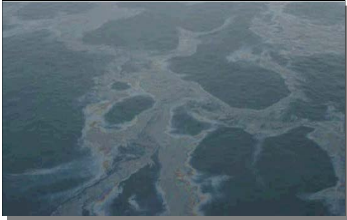
Figure 10: A photograph showing the difference between silvery sheen and rainbow sheen oil around the edges. The thickness of the silvery sheen is between 0.04 \text{ g/m}^2 – 0.3 \text{ g/m}^2 . The thickness of the rainbow sheen is 0.3 \text{ g/m}^2 – 5.0 \text{ g/m}^2 (source: Bonn Agreement Aerial Surveillance Handbook, 2004 – Part 3, Annex A).
