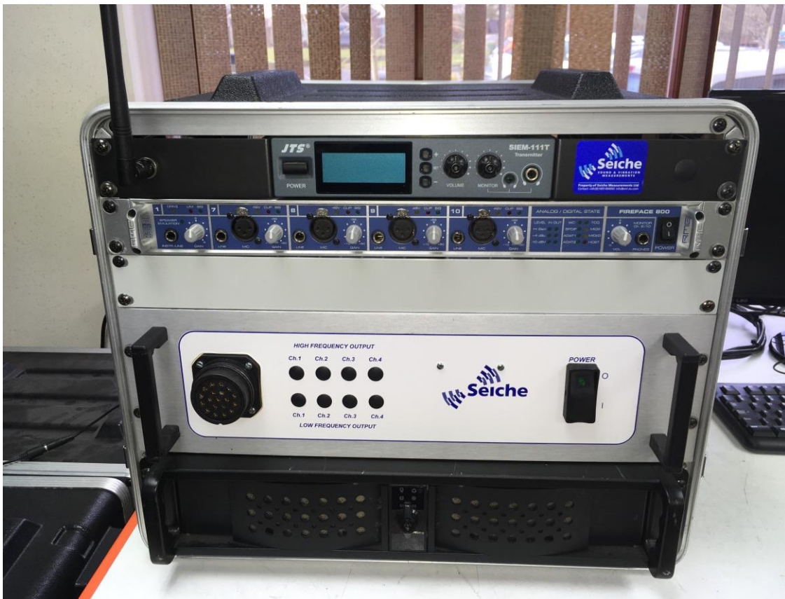
Figure 3: Electronic 8U base unit including PC and LF and HF monitors
