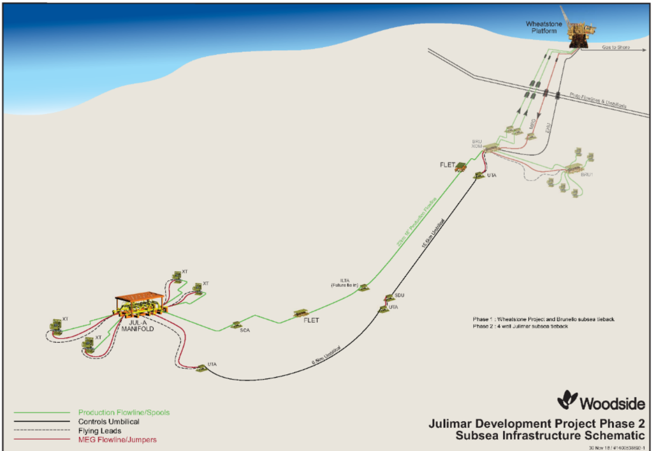
Figure 3-1: Generalised schematic of Julimar Development Project Phase 2
