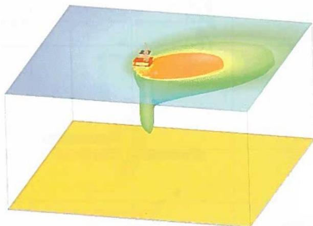
**Figure 5-1 Schematic diagram of the modelled PFW discharge from Esso's Kingfish B platform (McAllister, 1997)**
