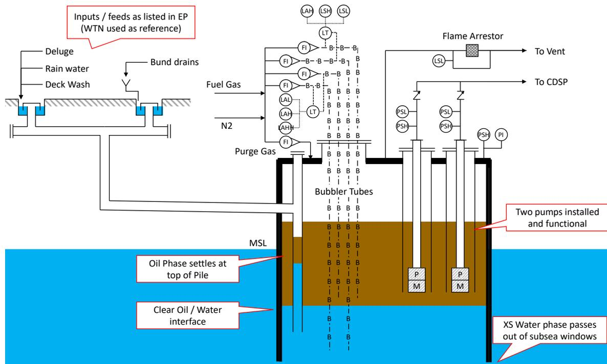
**Figure 6-2 Pile System Schematic**
