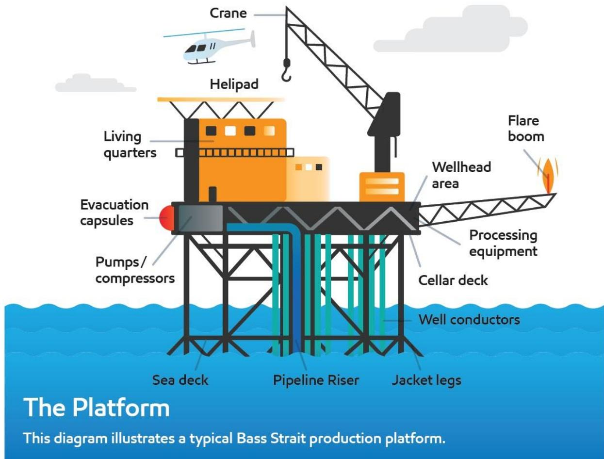
Figure 2-2 Schematic - Bass Strait Oil and Gas Platform
