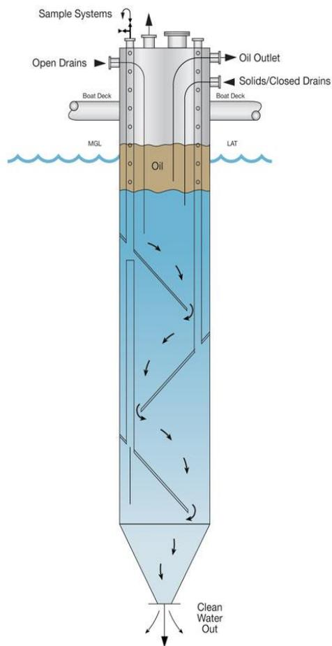
**Figure 2-3 Generic diagram of pile system**
