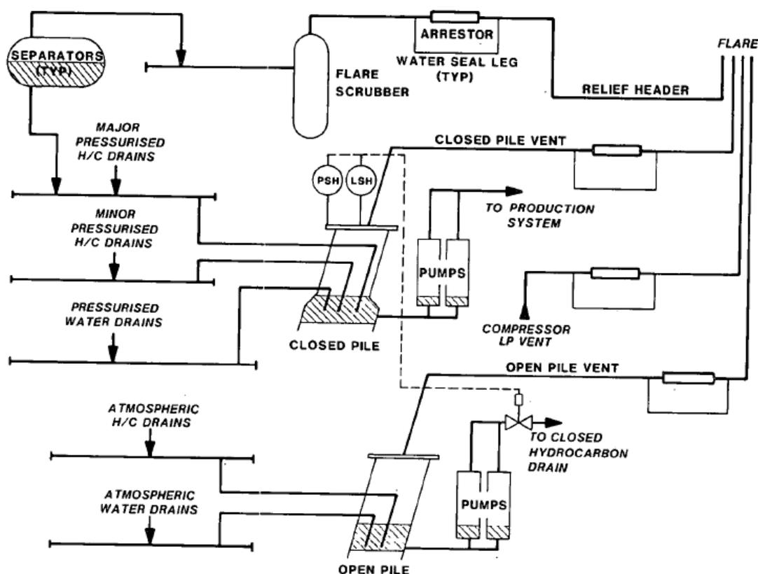
**Figure 2-4 Generic Flare Vent & Drain Model**
