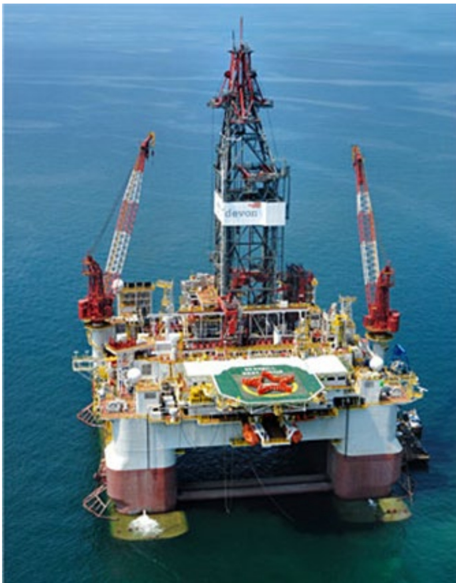
Figure 6.1 Typical MODU, Seadrill's Limited's West Sirius
