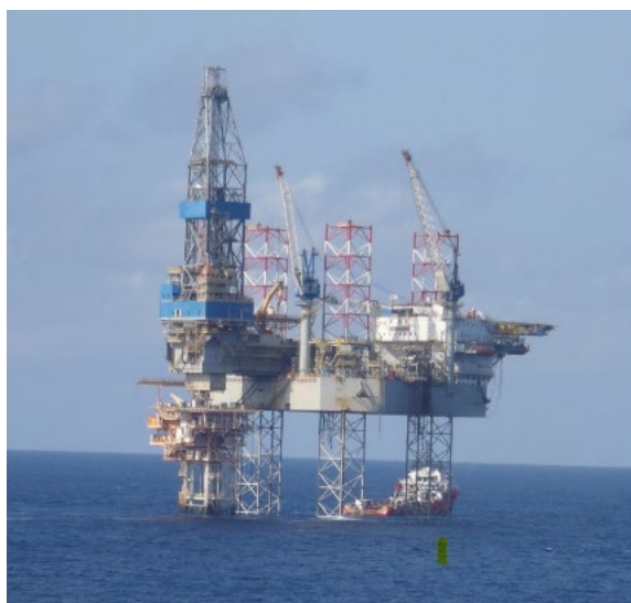
Figure 2-2: Positioning the MODU alongside a Wellhead Platform
