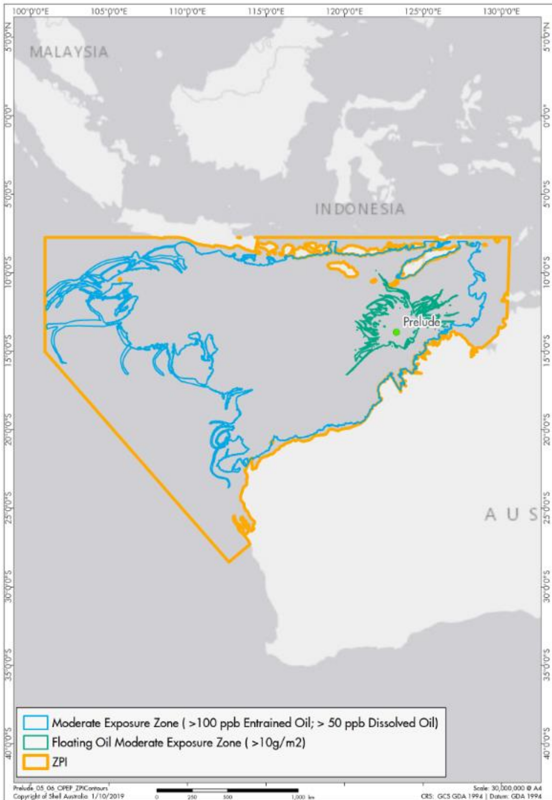
Figure 9-22: Extent of the ZPI (low exposure threshold) and the moderate exposure thresholds (floating, dissolved and entrained) based on the stochastic results of all worst case credible spill scenarios combined
