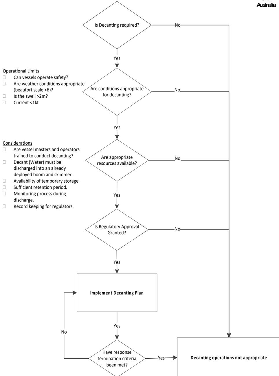
**Figure 10-2: Shell Decanting Response Guide**
