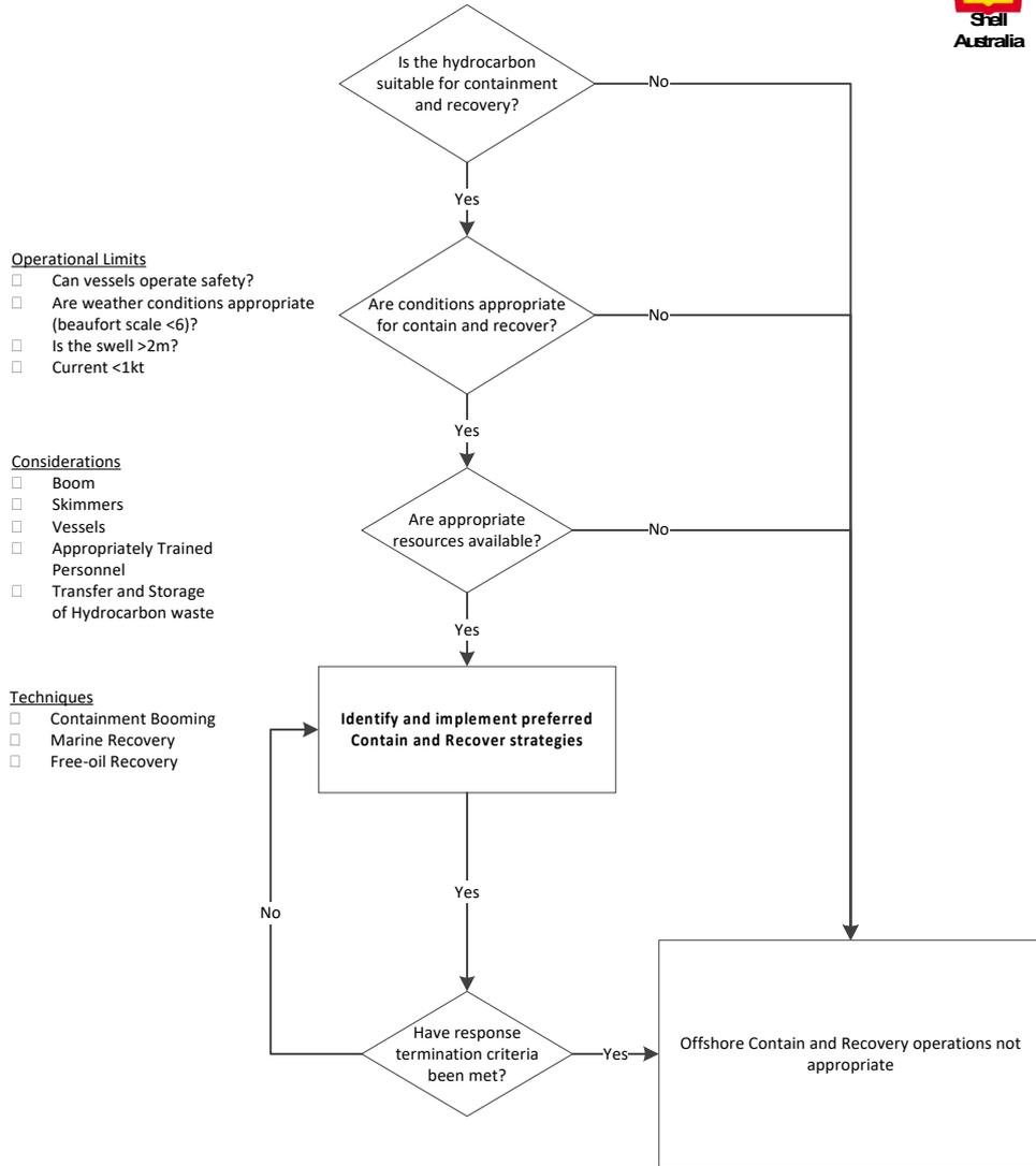
**Figure 10-1: Shell Offshore Contain and Recover Guide**
