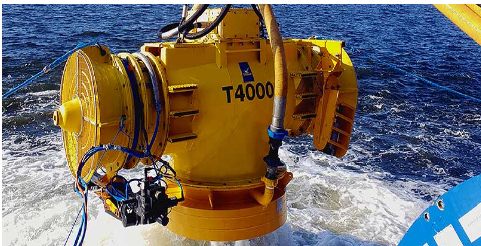
Figure 3-6: Example of equipment used for mass flow excavation
