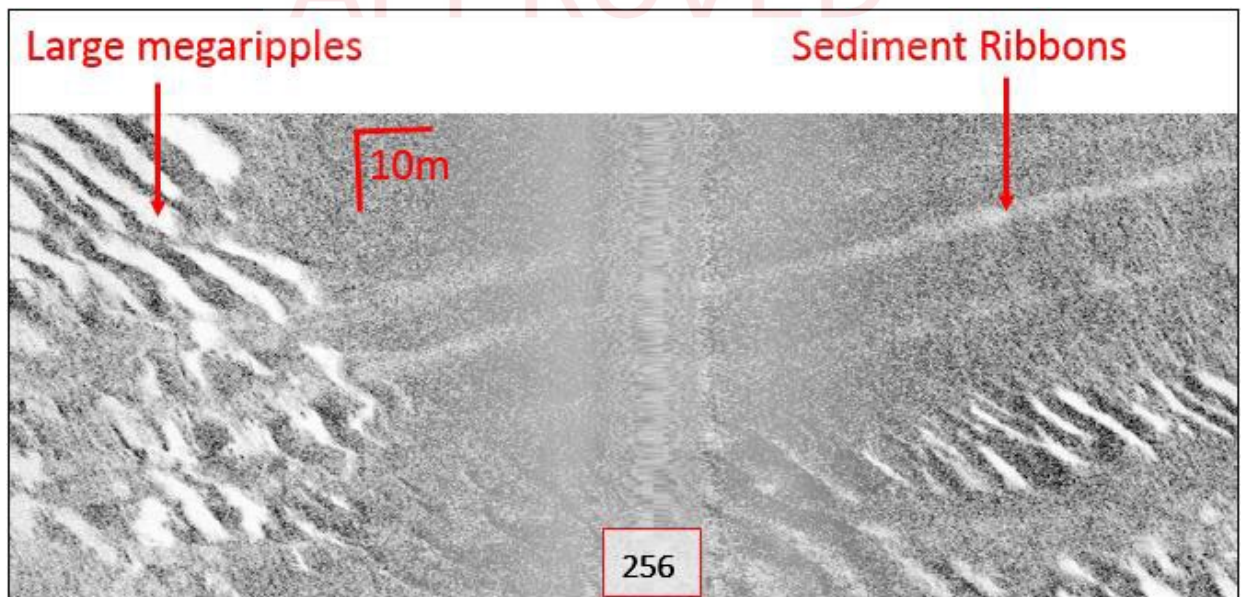
Figure 4-27: SSS image from KP256 showing large megaripples and sand ribbon lineations indicating significant currents
