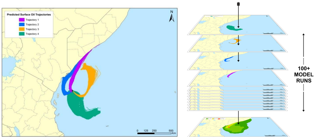
Figure 5.1 Predicted movement of four single oil spill simulations by SIMAP for the same scenario (left image). All model runs are overlain (right image) and the number of times that trajectories contact a given location at a concentration is used to calculate the probability (Source: NOPSEMA, 2018).
