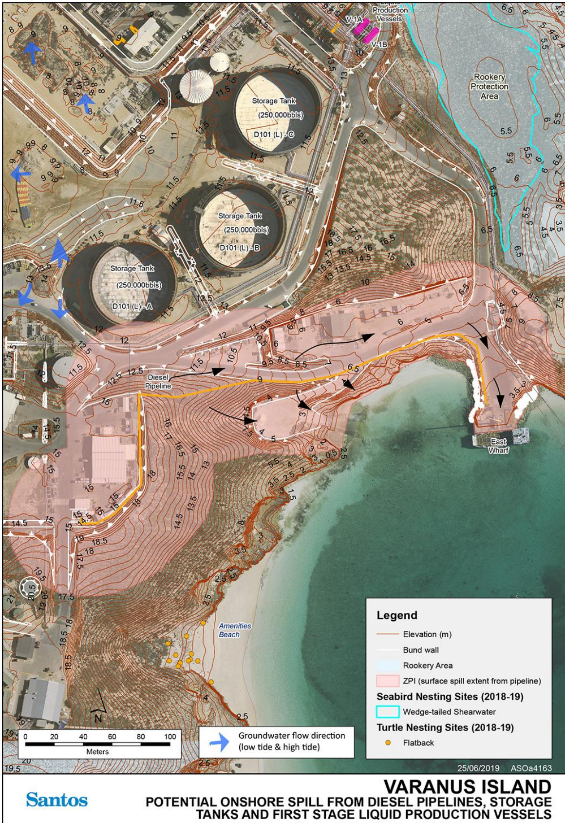
Figure 3-4: Onshore pipelines (Diesel) spill ZPI - surface
