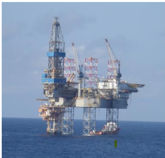
Figure 2-2: Positioning the MODU alongside a Wellhead Platform
