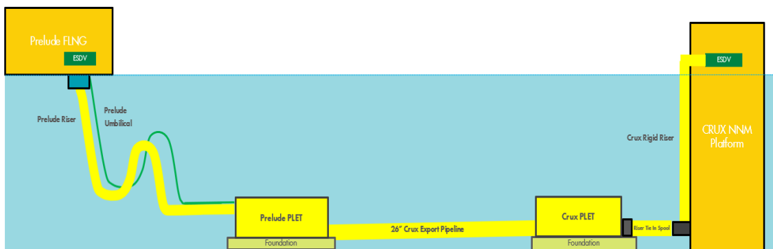
Figure 5-6: Export Pipeline and Subsea Integration System
