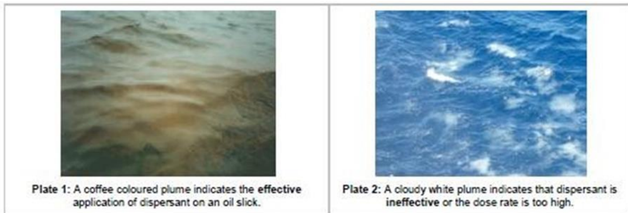
Figure 10-1: Effective and Ineffective Dispersant Application
