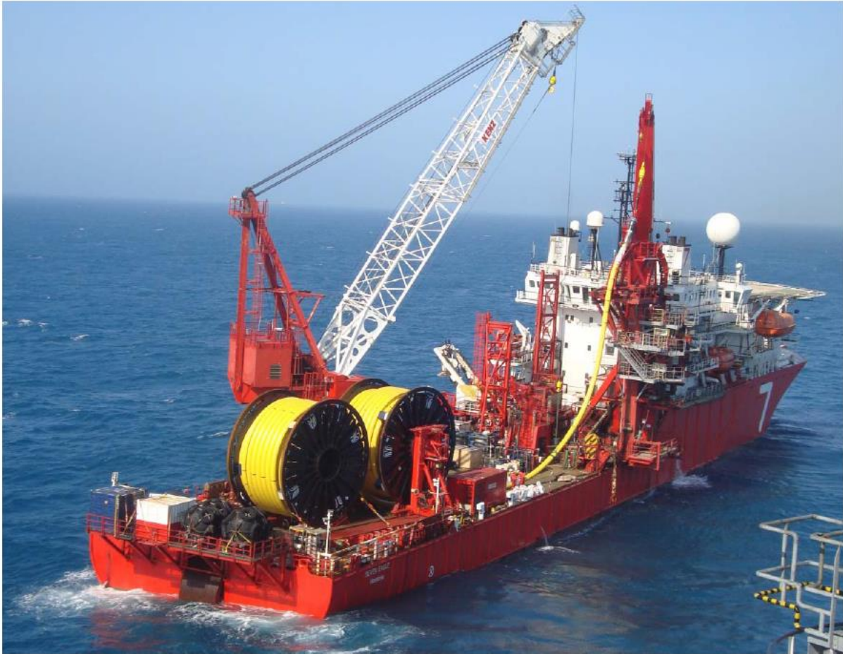
Figure 2-14 Multi-Purpose DSV Seven Eagle
