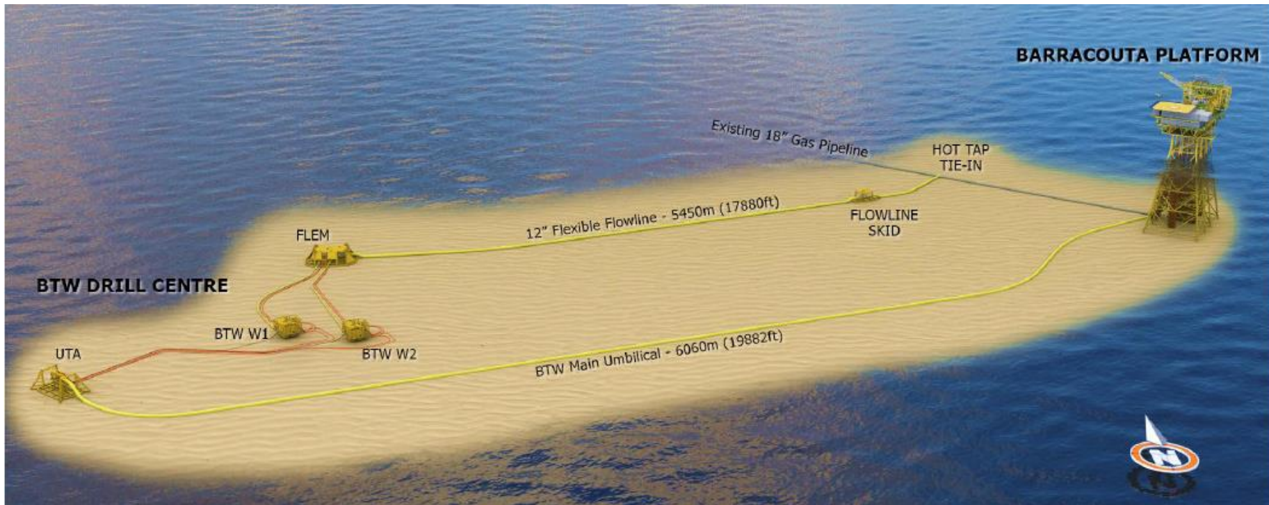
Figure 2-4 Indicative BTW Field Layout
