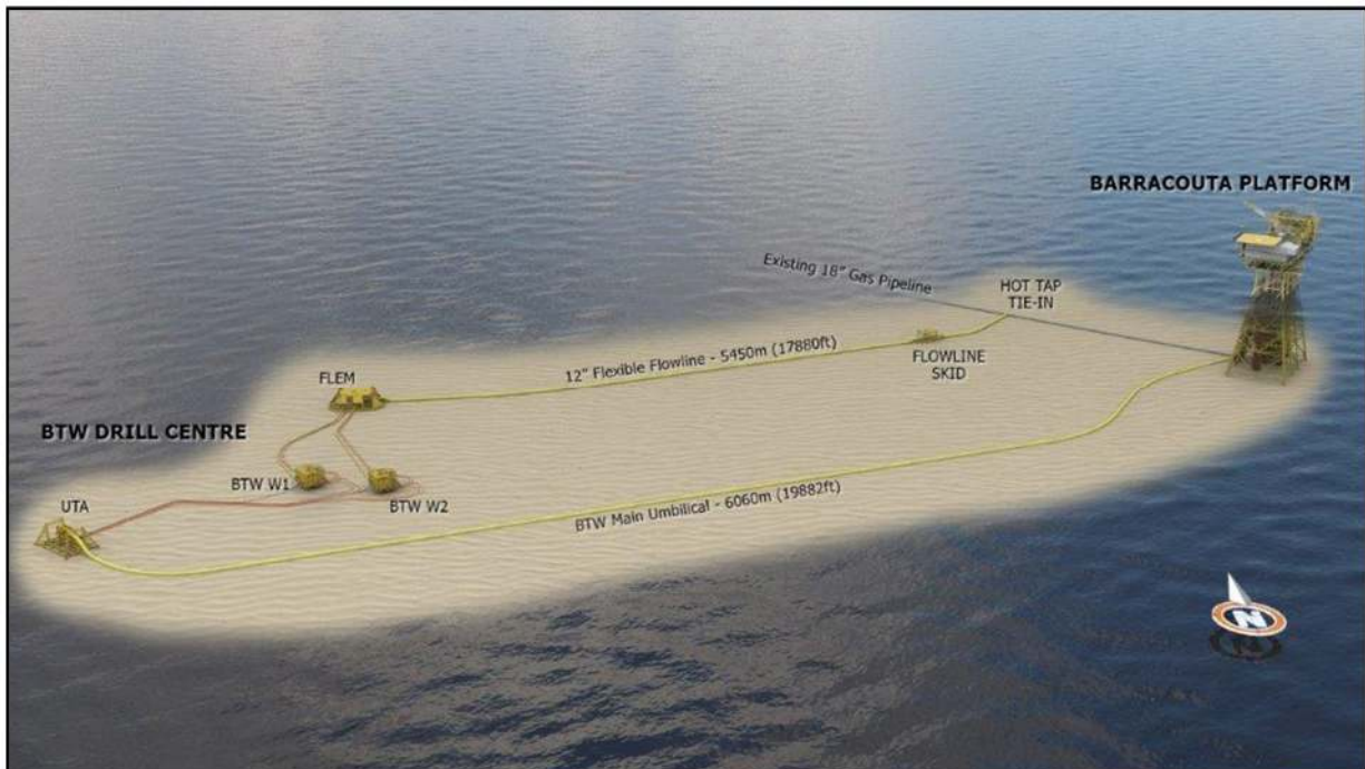
West Barracouta (BTW) Field Development Schematic
