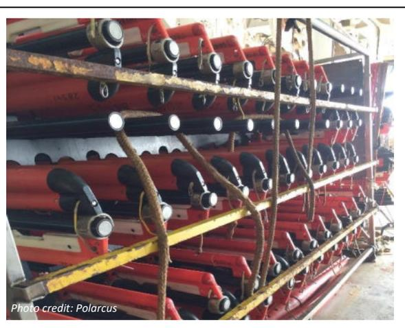
**Photo 2.4: Tail buoy (with navigation light at top)**
