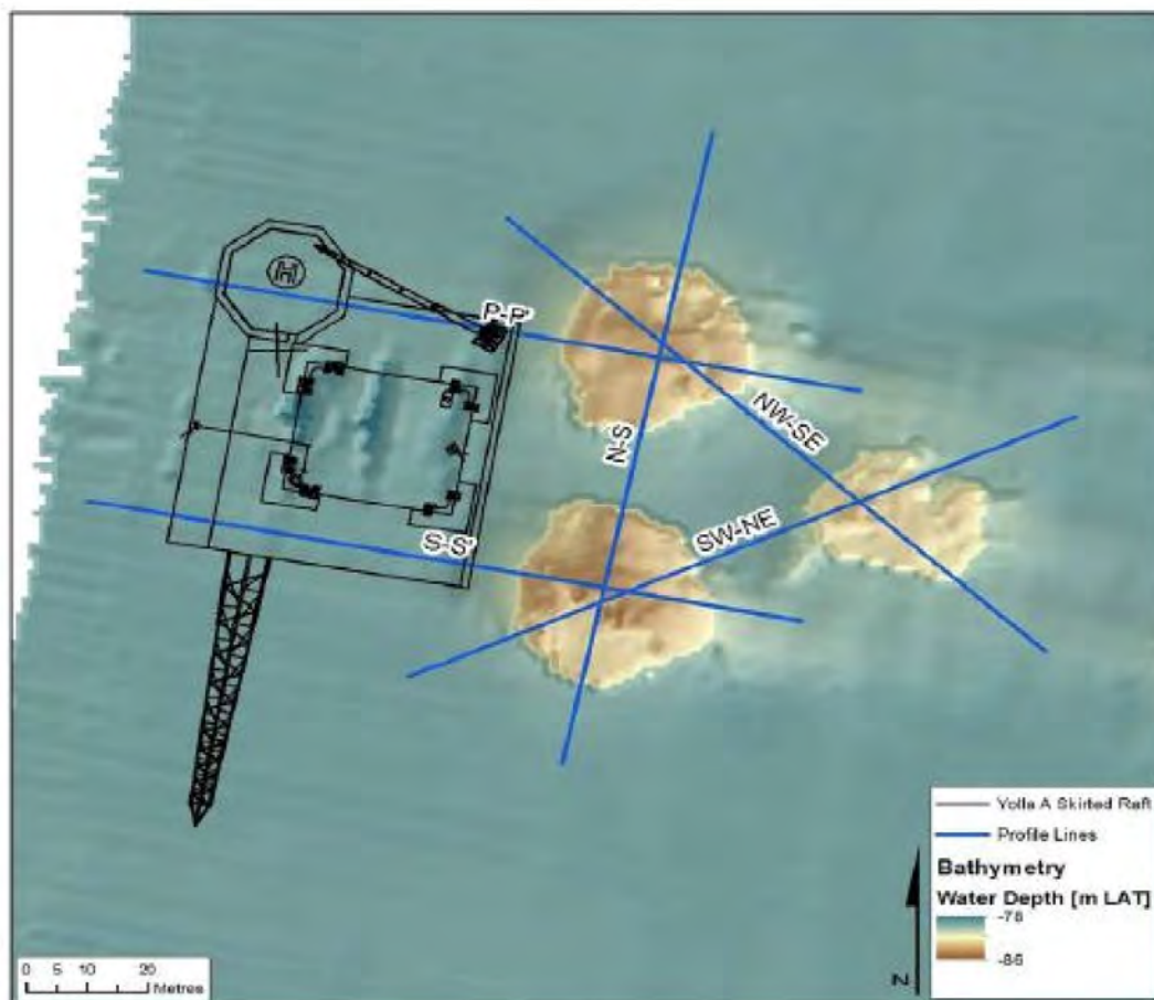
Figure 5.9. Existing drill rig spud can depressions on the east side of the Yolla platform
