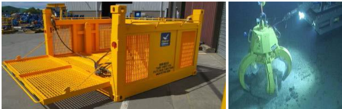
Figure 3-20: Bespoke recovery basket (left) and grab (right)
