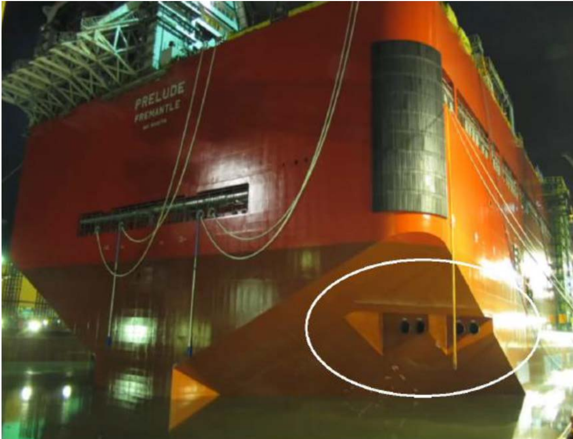
Figure 9-8: View of cooling water discharge ports P53, P54 (inboard pair), P63 and P64 (outboard pair) that discharge rearwards on the starboard side
