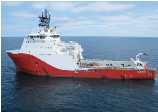
Figure 7. Photo of a Siem Anchor Handling Tug Supply (AHTS) vessel (Siem Offshore 2010).
