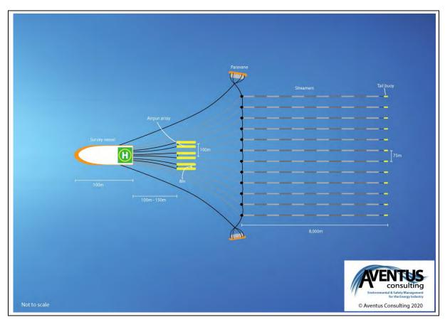
Figure 3.7. Plan view of a typical MSS arrangement
