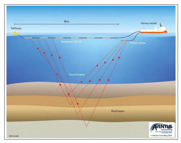
Figure 3.4. Profile view of a typical MSS arrangement
