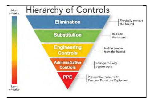
Figure 6.3. The Hierarchy of Controls
