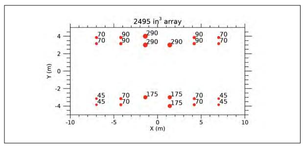
Figure 3.5. Anticipated airgun arrangement for the Prion 3DMSS
