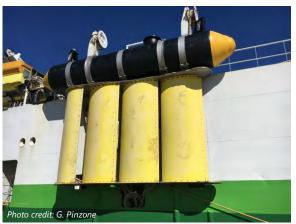
Photo 3.4. Tail buoy (with navigation light at top)
