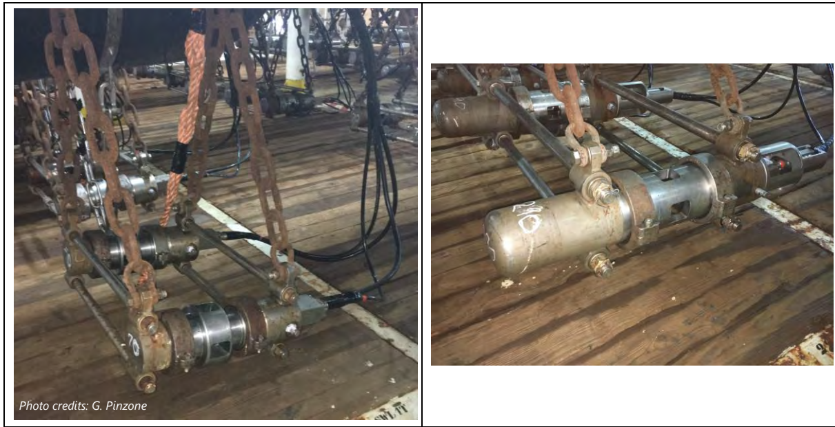
Photo 3.1. Typical airgun used for a 3DMSS (as part of the array, and close up)
