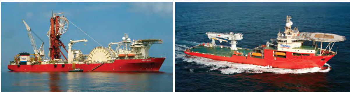
Figure 3. Photos of Deep Blue (Technip 2012) and Deep Orient (Technip 2013), the pipelay and construction vessels used as proxy for the Project pipelay and installation vessel.
