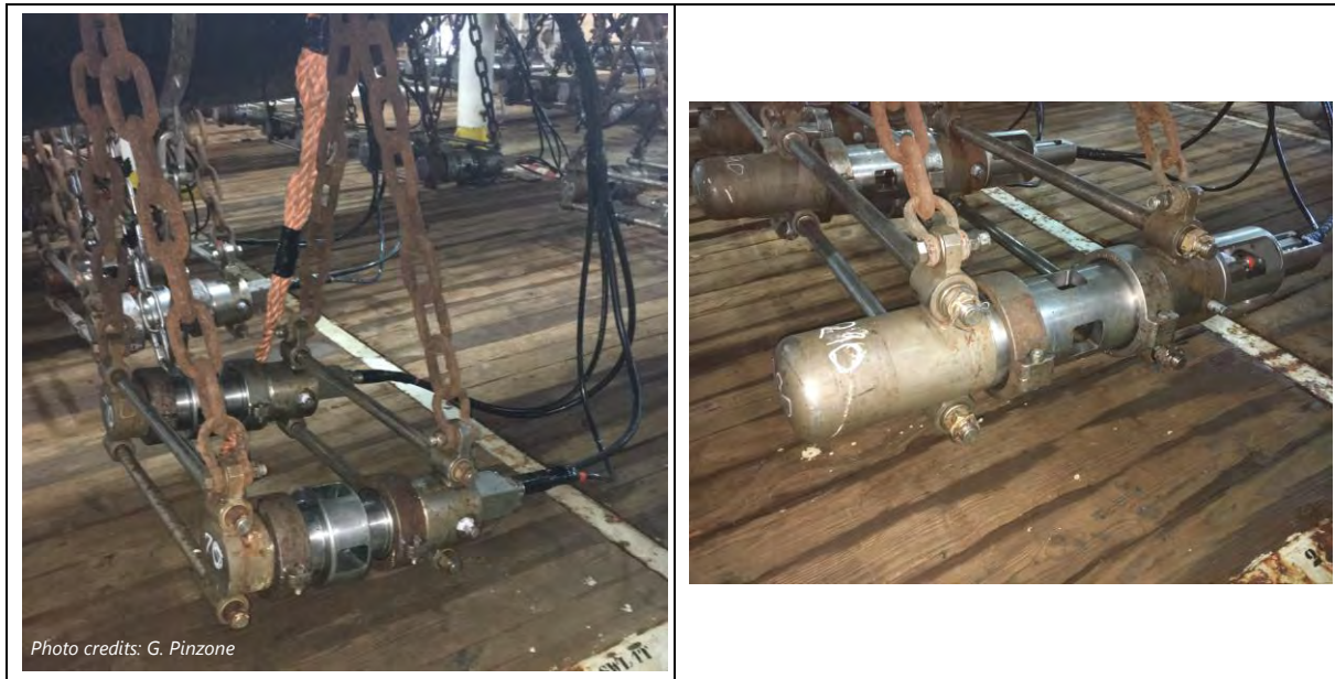
Photo 3.1. Typical airgun used for a 3DMSS (as part of the array, and close up)
