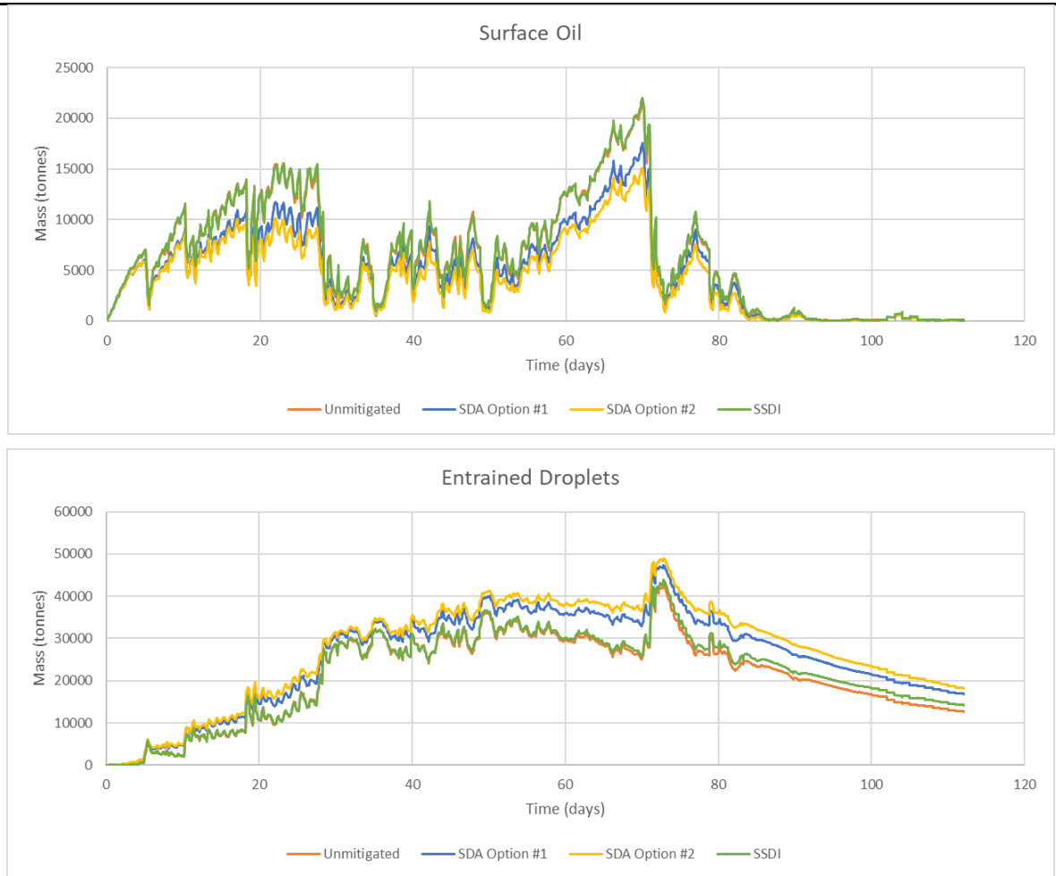
Figure 8-7 Comparison of no dispersant (orange), SDA (blue) and SSDI (green) response strategies on the mass of surface oil (top) and entrained droplets (bottom)
