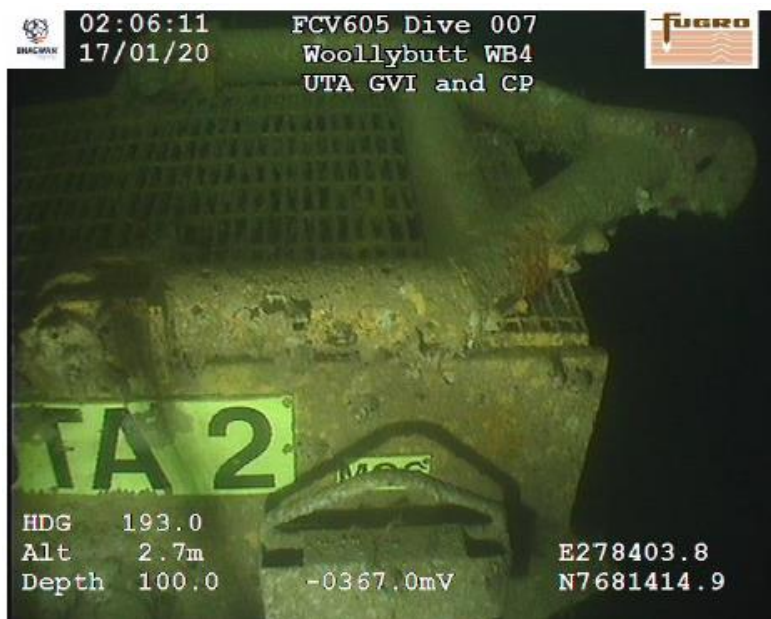
Figure 3-13: WB4 UTA lifting arm
