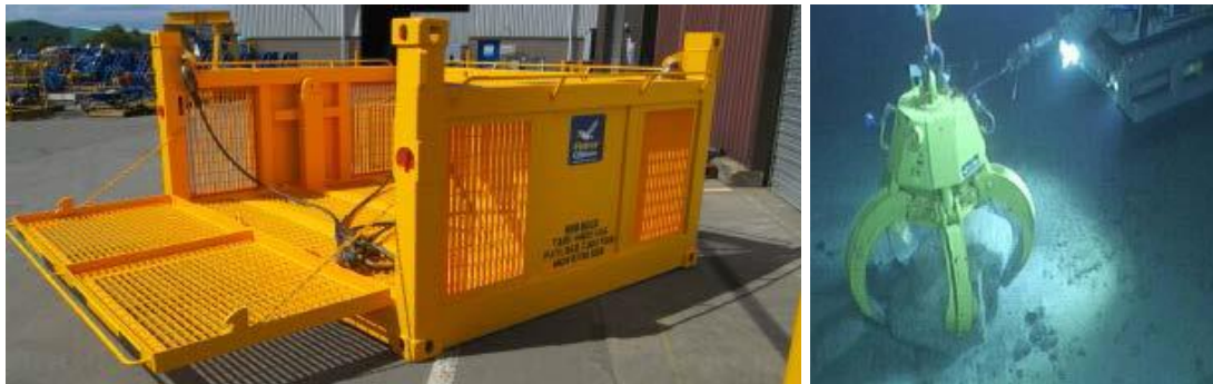
Figure 3-24: Bespoke recovery basket (left) and grab (right)
