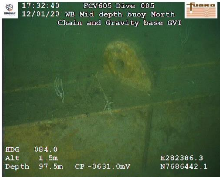
Figure 3-21: North MDB gravity base padeye
