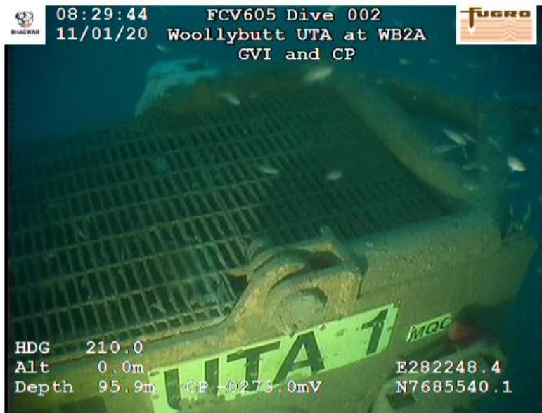
Figure 3-12: WB2A UTA lifting arm
