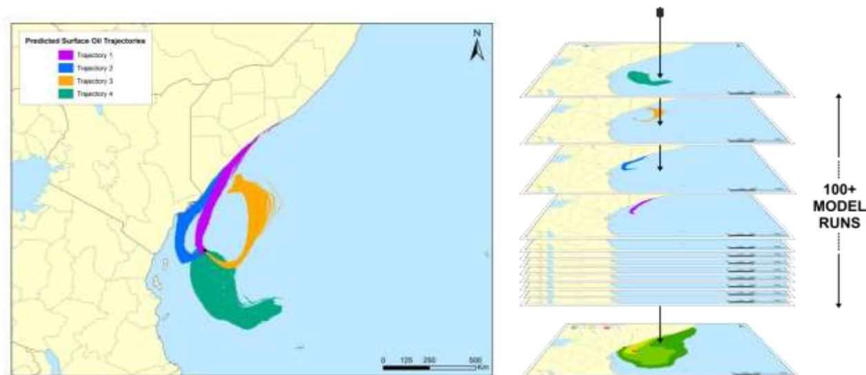
Figure 7.1 Predicted movement of four single oil spill simulations by SIMAP for the same scenario (left image). All model runs are overlain (shown as the stacked runs on the right) and the number of times that trajectories contact a given location at a concentration is used to calculate the probability (Source: NOPSEMA, 2018).
