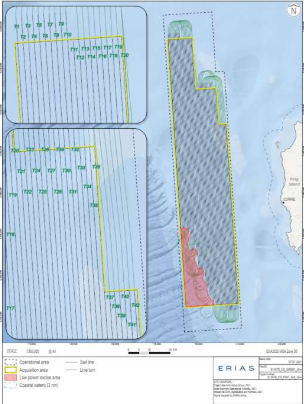
Figure 4-41: Acquisition lines for adaptive planning (Note: Sail-lines shown are indicative only and line run-ins and run-outs will not occur outside of the acquisition area.)
