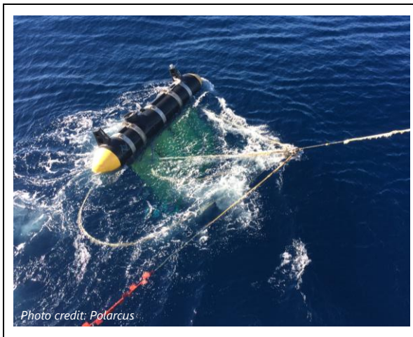
Photo 3.6. Paravane being launched
