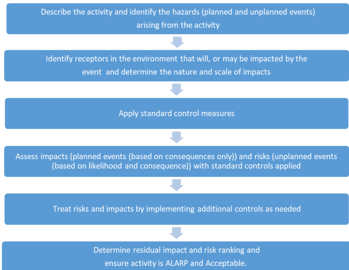
Figure 5-1: Hazard Identification and Assessment Guideline
