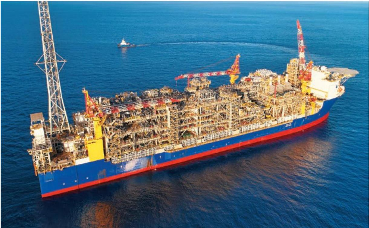
**Figure 3-5: The floating production, storage and offtake (FPSO) facility**
