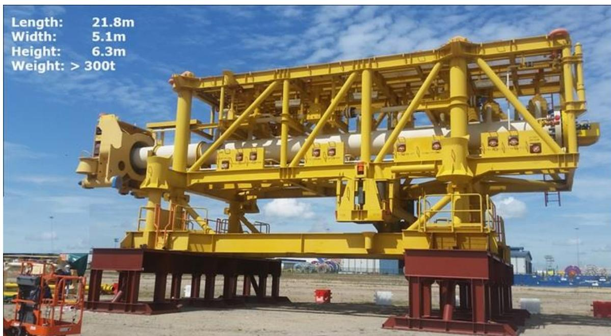
**Figure 3-8: Pig launcher receiver**
