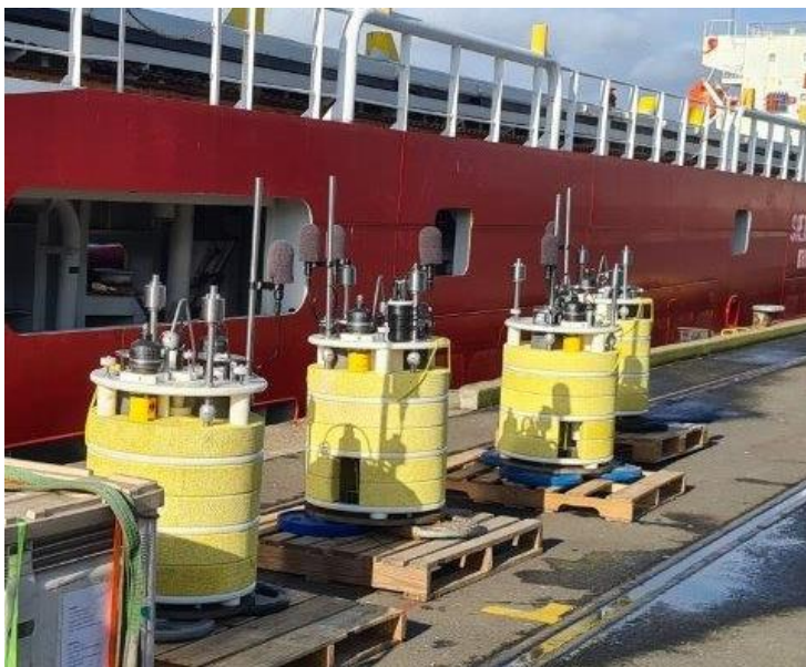
Figure 10. The four C-Lander bottom moorings with Autonomous Multichannel Acoustic Recorders (AMAR G4s; JASCO) used for the project prior to loading onto the Siem Sapphire .
