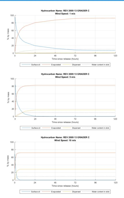
Figure 6-1 Simulated weathering of the SINTEF REV 2009 13 GRADER C hydrocarbon for constant wind speeds of 1 m/s (top), 5 m/s (middle) and 10 m/s (bottom) (GHD, 2020a)
