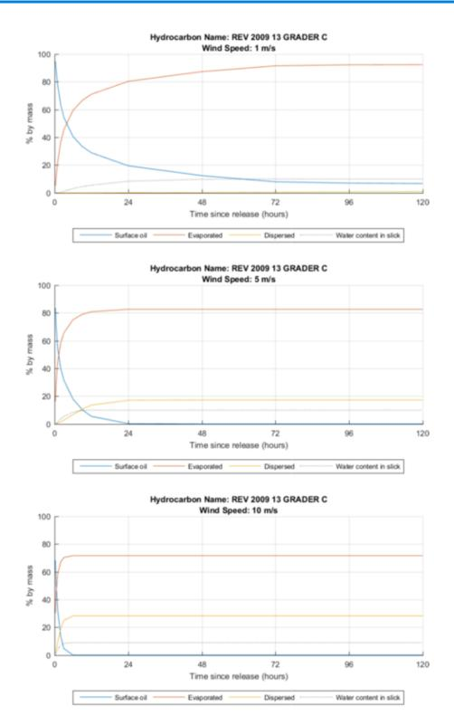
Figure A 2: Simulated weathering of the SINTEF REV 2009 13 GRADER C hydrocarbon for constant wind speeds of 1 m/s (top), 5 m/s (middle and 10 m/s (bottom) (GHD, 2020b)
