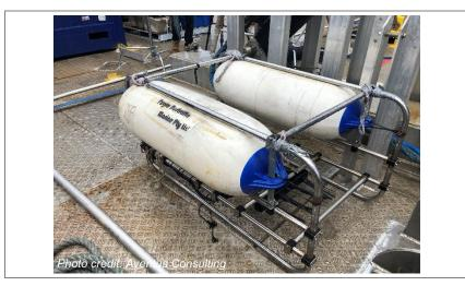
Photo 2.5 Example shallow seismic sound source
