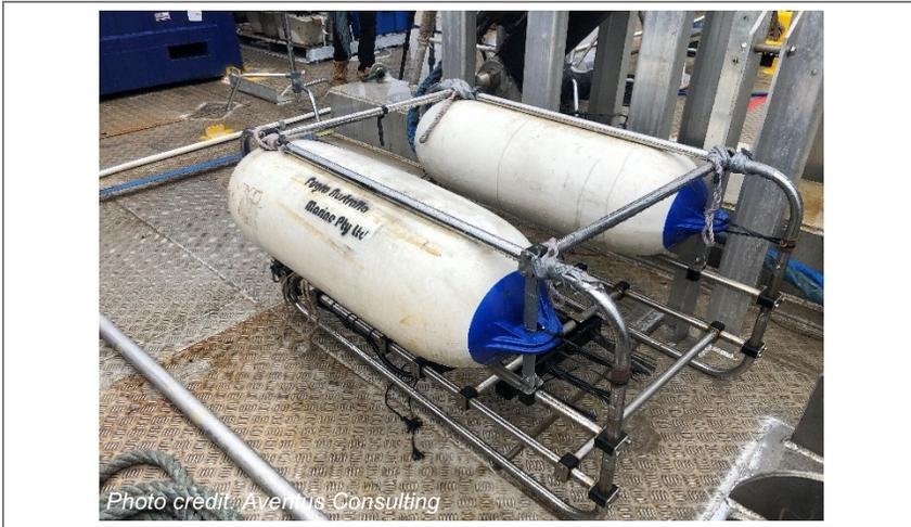
**Photo 2.5** Example shallow seismic sound source
