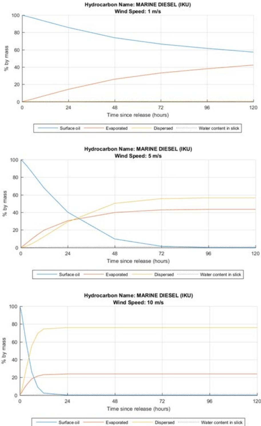
**Figure 7-6: Simulated Weathering of the Foundation for Specific and Industrial Research at the Norwegian Institute of Technology (SINTEF) Marine Diesel (IKU) Hydrocarbon for Constant Wind Speeds of 1 m/s (top), 5 m/s (middle) and 10 m/s (bottom)**
