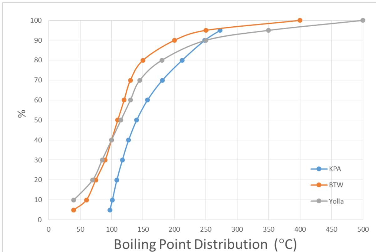
**Figure 6-5 Boiling Point Distribution of Representative (Yolla), KPA Condensates**
