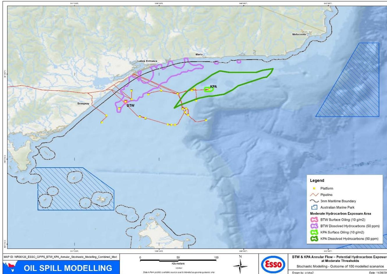
Figure 6-7 Discharge Scenario 1 Annular Flow LOWC condensate spill stochastic modelling output for KPA release location. Hydrocarbon exposure at the moderate thresholds (Surface: 10 g/m<sup>2</sup> and In-water (dissolved): 50 ppb instantaneous)
