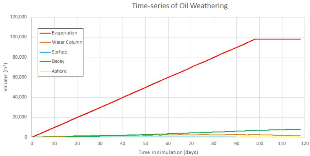
**Figure 6-6** Predicted weathering and fates graph as volume for the selected single KPA LOWC trajectory: largest surface swept area
