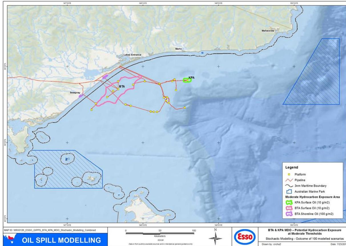
Figure 6-3 Vessel collision MDO spill stochastic modelling output for KPA release location. Hydrocarbon exposure at the moderate thresholds (Surface: 10 g/m<sup>2</sup>)
