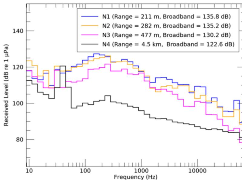
Figure 5-3 Overview Received levels (RL) for Skandi Feistein and MMA Leeuwin operating at the KFB platform during 2021-04-14 from all four monitoring stations (Jasco, 2021)
