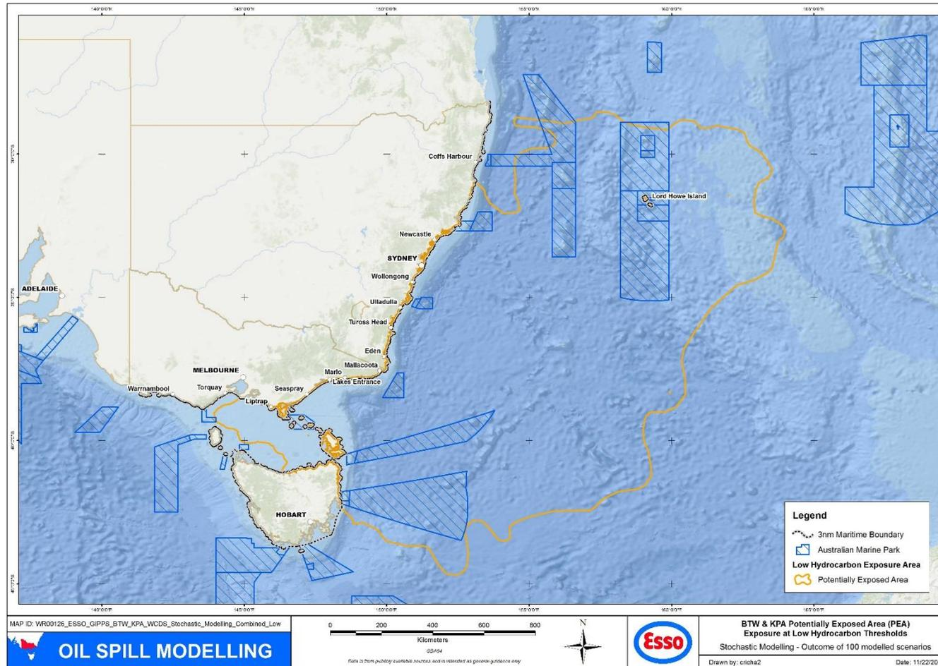
**Figure 4-1 Potentially Exposed Area – Stochastic modelling LOWC WCDS Open Hole (combined outcome of 100 modelled scenarios) showing instantaneous contact at lowest hydrocarbon thresholds (10ppb instantaneous entrained).**
