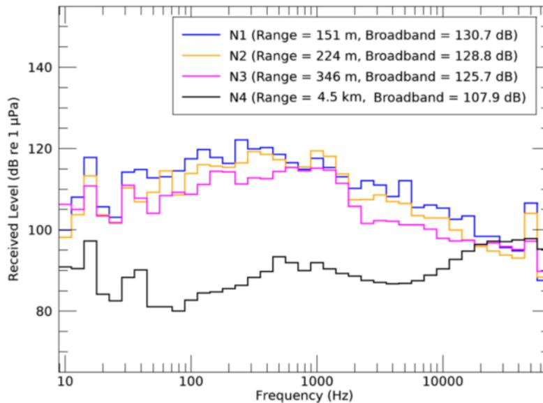
Figure 5-2 Received levels (RL) for the Skandi Feistein and MMA Leeuwin operating at the BTA platform during 2021-03-27 from all four monitoring stations (Jasco, 2021)
