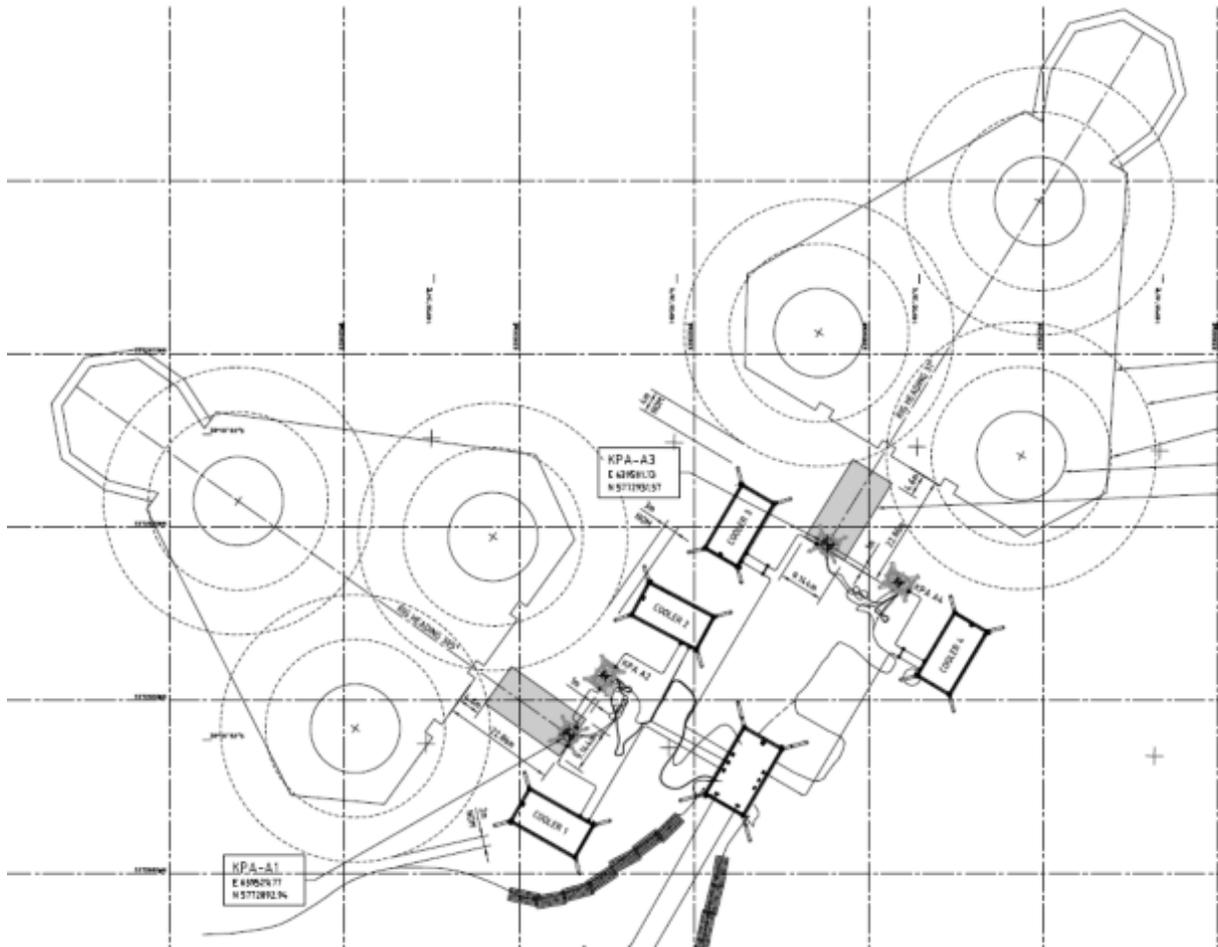
Figure 6-4 Jack-up positioning above KPA facilities
