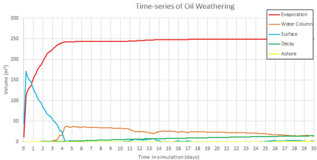
**Figure 6-2** Predicted weathering and fates graph as volume for the selected single KPA MDO spill trajectory: largest surface swept area.
