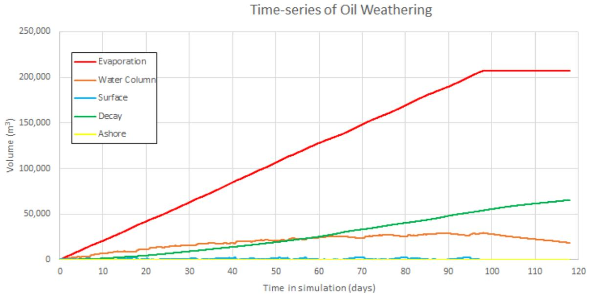
**Figure 6-8** Predicted weathering and fates graph as volume for the selected single KPA LOWC trajectory: largest volume ashore and longest length of actionable oil on the shoreline (above 100 g/m<sup>2</sup>)
