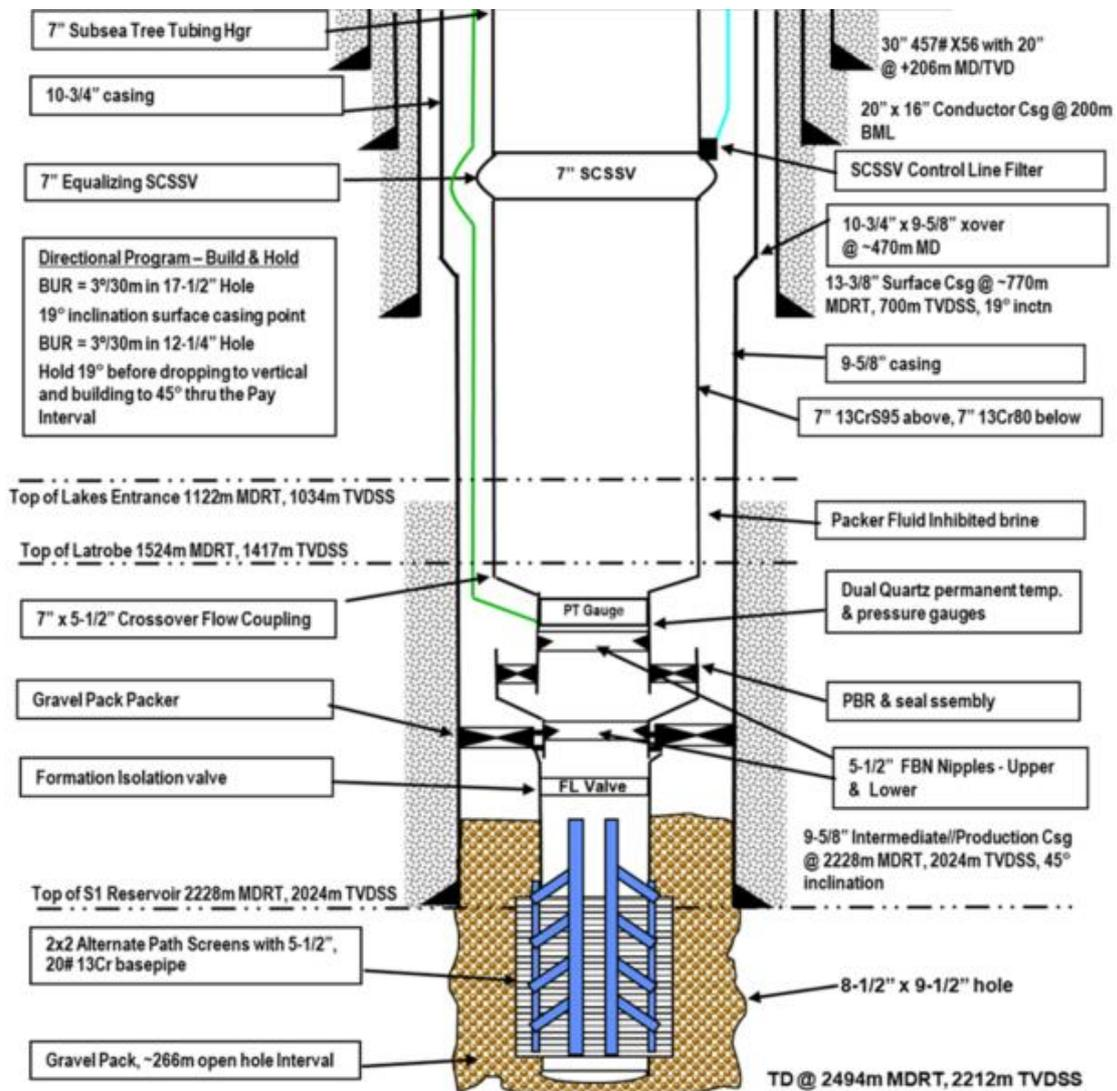
**Figure 2-3 KPA Well Schematic**
