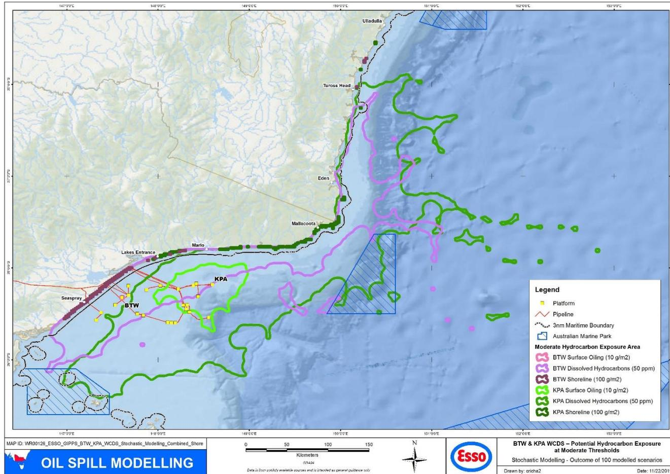
Figure 6-9 Discharge Scenario 2 Open Hole LOWC condensate spill stochastic modelling output for KPA release location. Hydrocarbon exposure at the moderate thresholds (Surface: 10 g/m<sup>2</sup>, Shoreline: 100 g/m<sup>2</sup> and In-water (dissolved): 50 ppb instantaneous)
