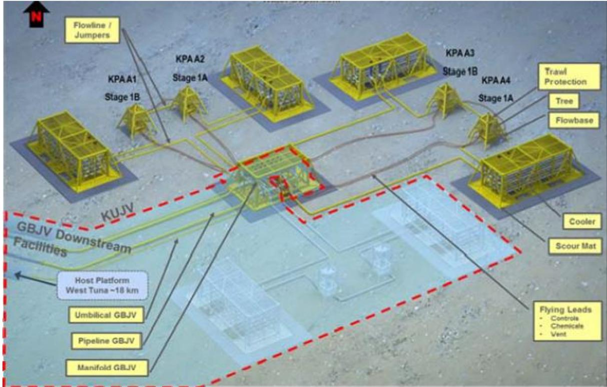
**Figure 2-2 KPA Subsea Facilities**
