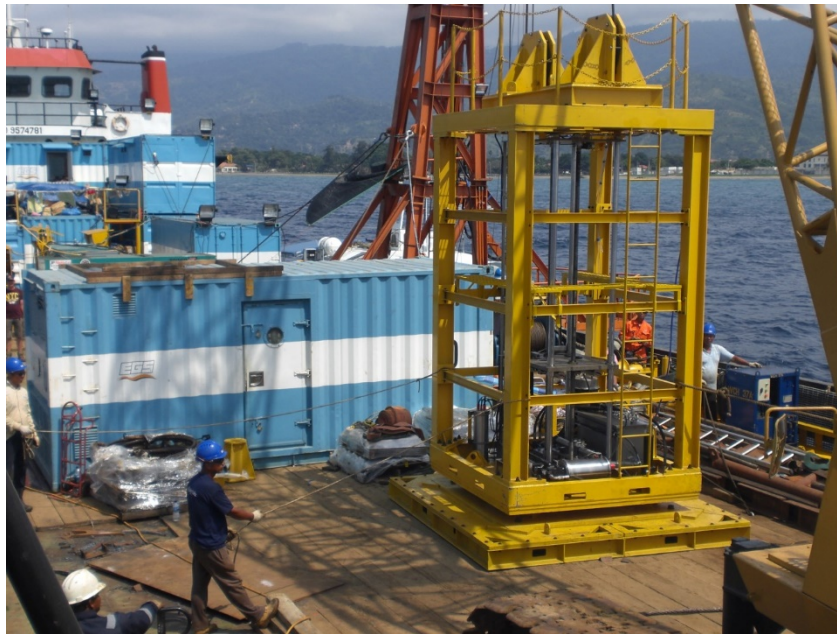
Photo 2.10. Standalone PCPT unit
