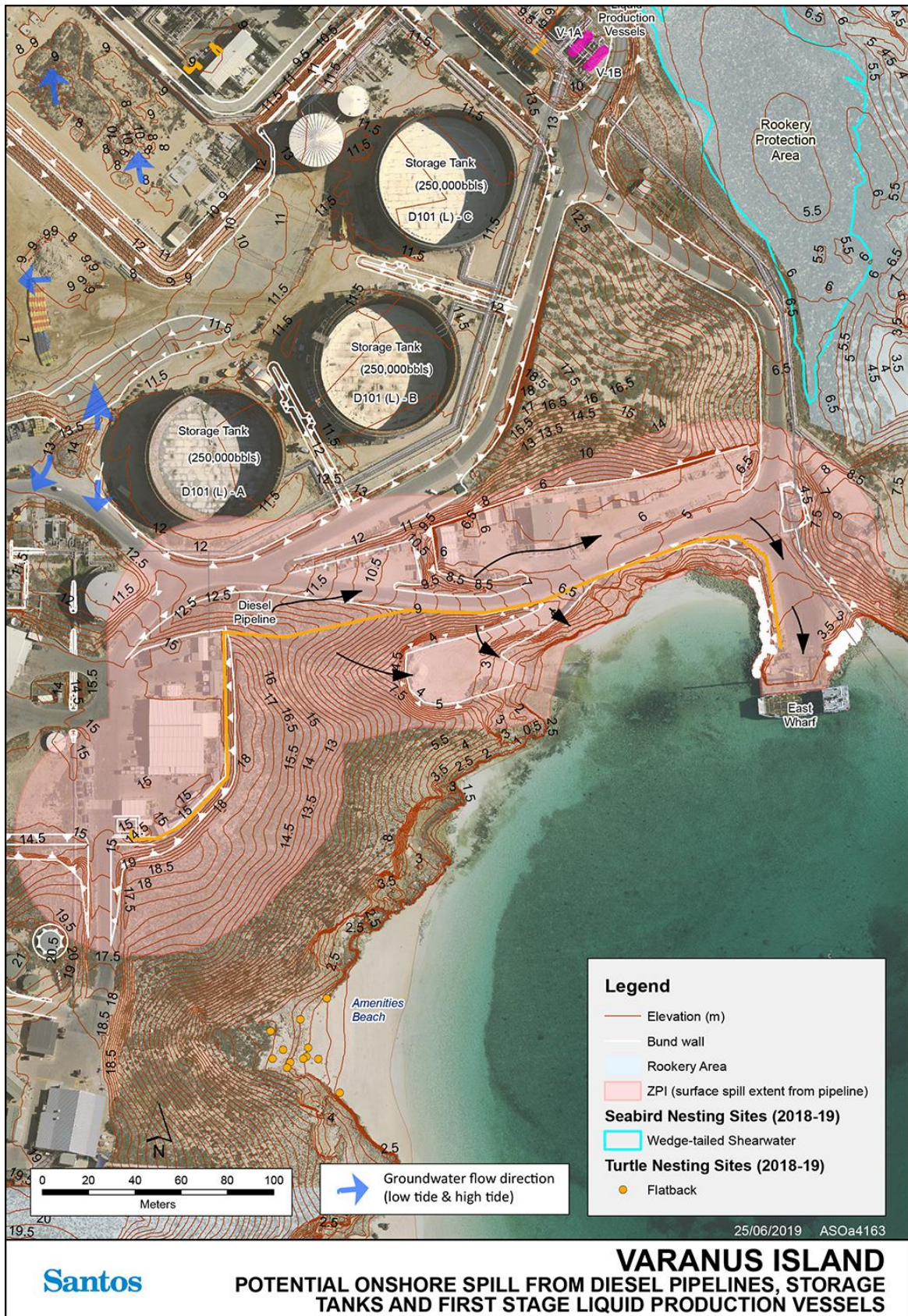
Figure 5-4: Onshore pipelines (Diesel) spill ZPI - surface
