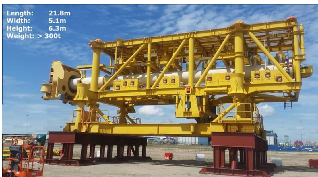
Figure 3-9: Pig launcher receiver
