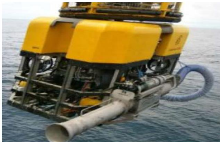
Figure 3-9: Typical ROV Mass Flow Excavator
