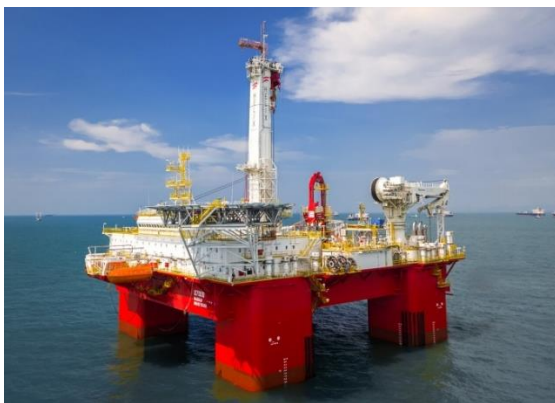
Figure 3. Well intervention unit Helix Q7000 semi-submersible platform (Helix Energy Solutions 2020).
