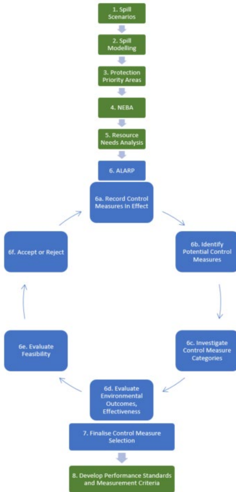
Figure B-1: ALARP Assessment Framework
