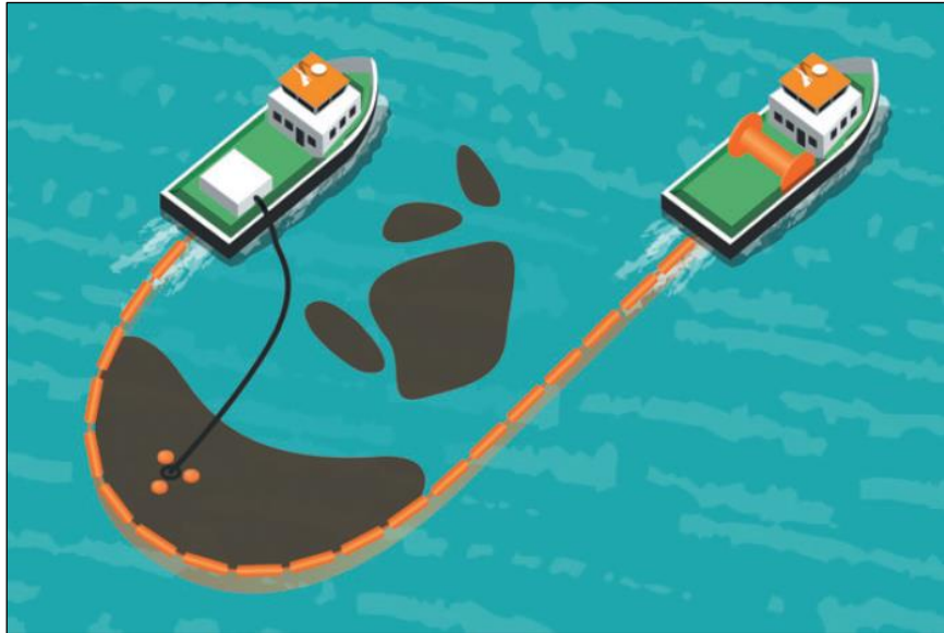
Figure 11-1: 'J' Configuration for Containment & Recovery Operations (Source: OSRL)
