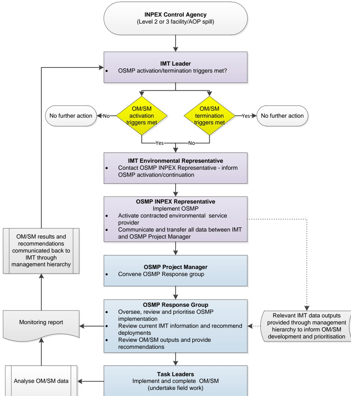
**Figure 4-6: OM and SM activation, termination and communication flowchart**
