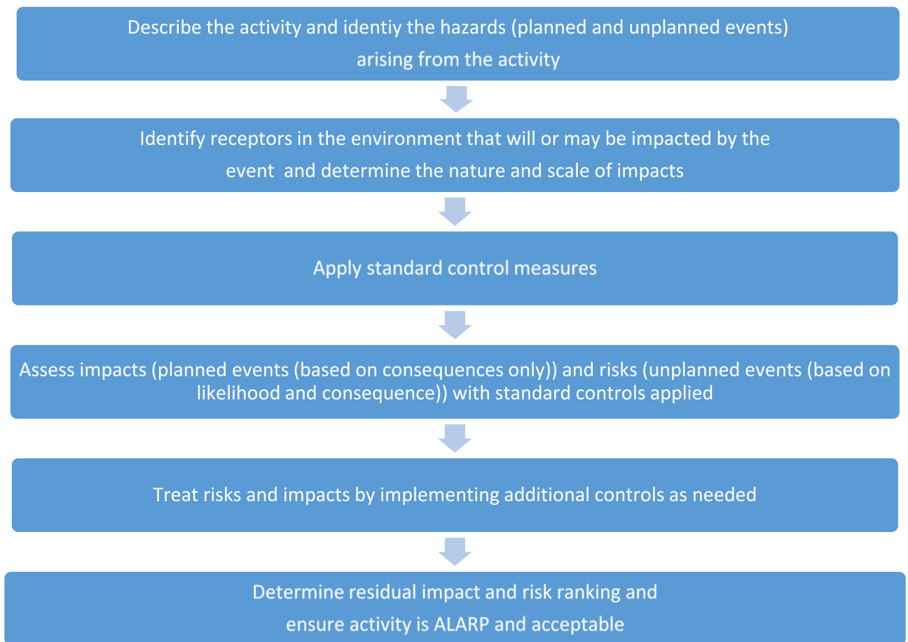
Figure 5-1 Environmental impact and risk assessment process
