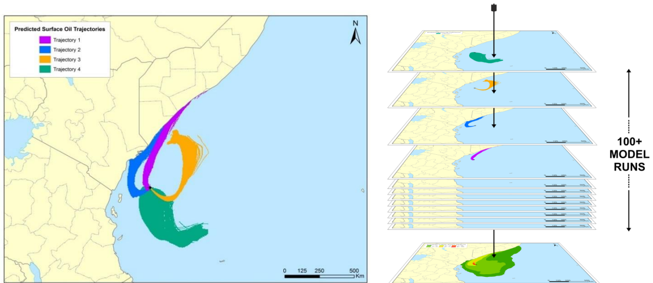
Figure 7.1 Predicted movement of four single oil spill simulations by SIMAP for the same scenario (left image). All model runs were overlain (right image) and the number of times that trajectories contact a given location at a concentration is used to calculate the probability (Source: NOPSEMA, 2018).
