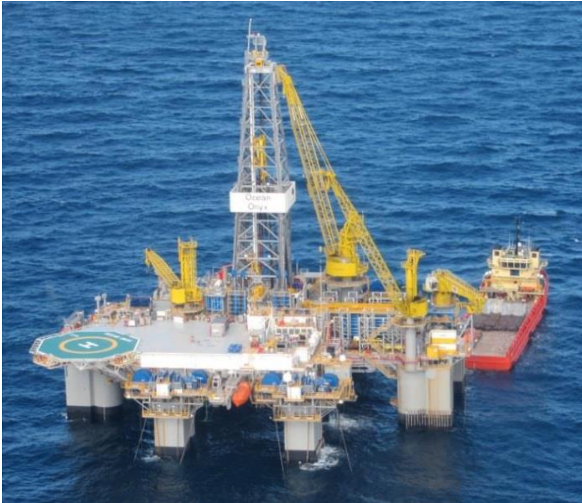
Figure 3. Ocean Onyx semi-submersible platform.
