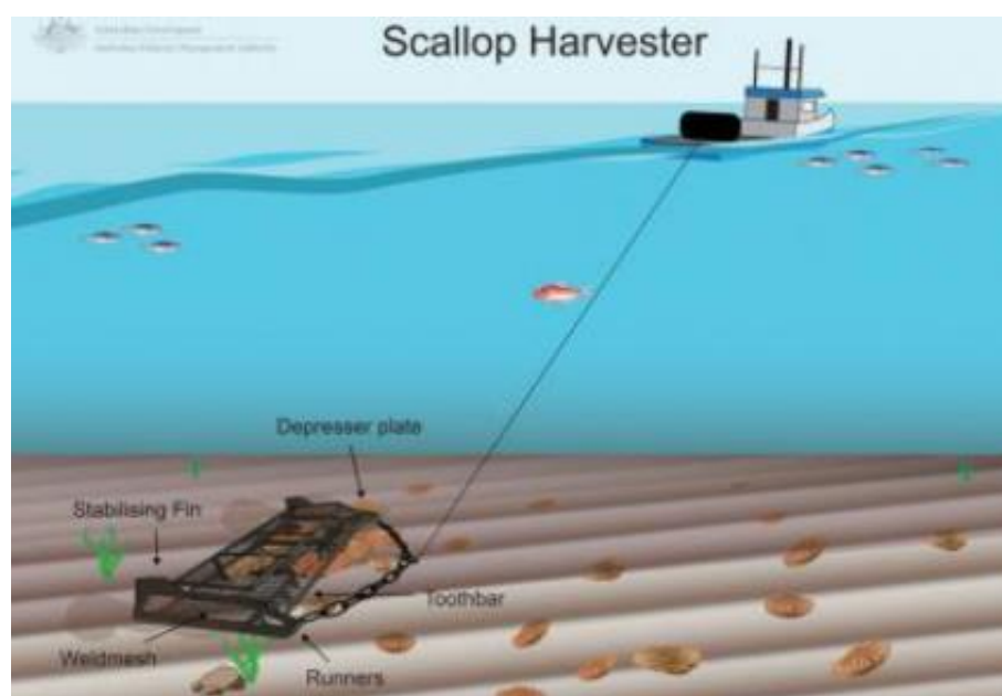
Figure 8-3 Scallop dredge main gear components
