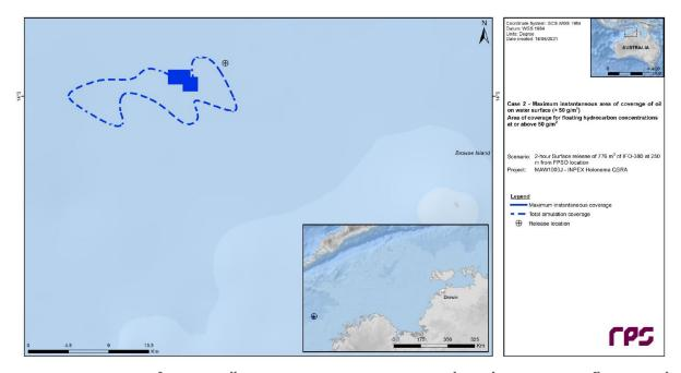
Figure 4-12: 776  $\mathrm{m}^3$  HFO spill maximum instantaneous, and total swept area floating oil  $>50\mathrm{g/m}^2$
