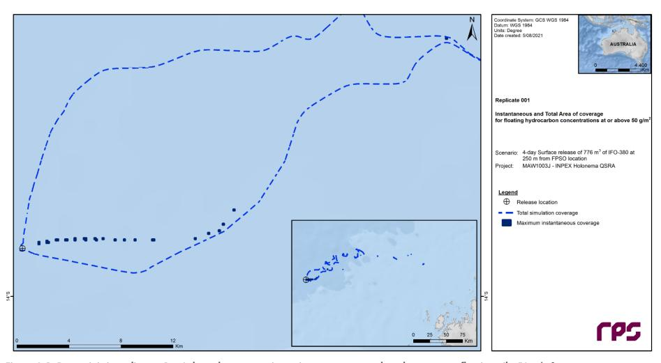
Figure 9-1: Deterministic replicate #1 – 4-day release – maximum instantaneous, and total swept area floating oil >50 g/m<sup>2</sup>
