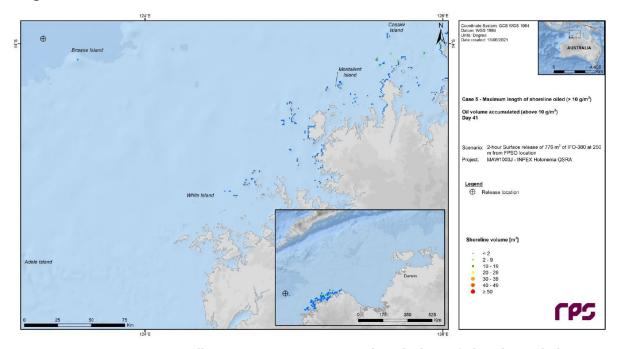
Figure 4-13: 776  $\rm m^3$  HFO spill instantaneous maximum length (km) of shoreline oiled at >10  $\rm g/m^2$ , showing instantaneous volumes oil ashore ( $\rm m^3$ )
