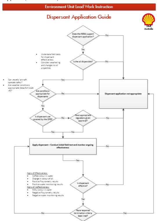
Figure 4-1: Shell Surface Dispersant Application Guide
