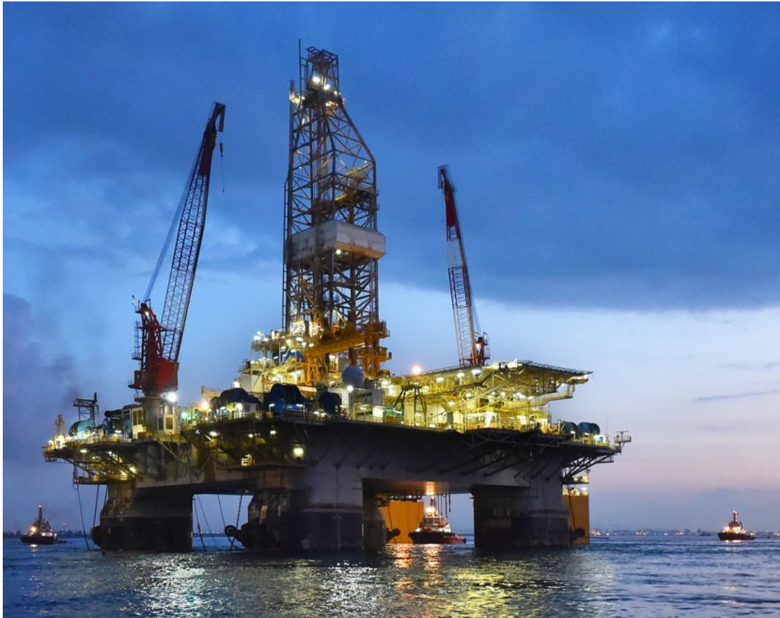
Figure 6-2: Representative Image of a Mobile Offshore Drilling Unit (the Valaris MS1)
